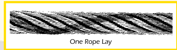
Figure 5: Lay as a Unit Measure
