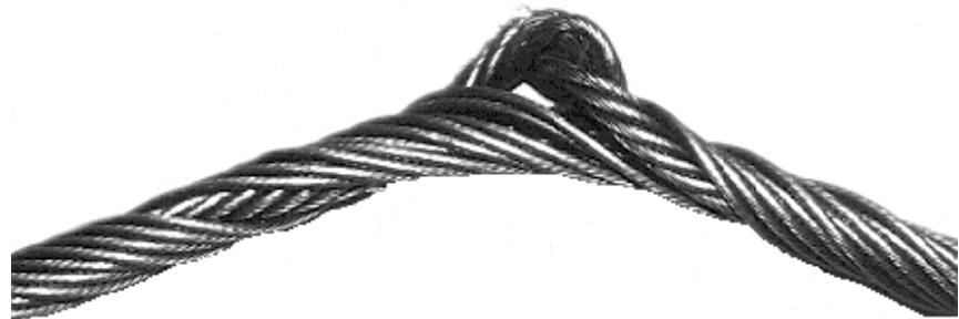
Improper installation procedures removed turns from this rope, loosening the outer strands and enabling the inner strands to protrude once the load was released.
