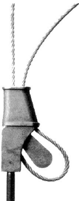
**Figure 8:** Seat the rope and wedge into the socket by quickly pulling the dead end
