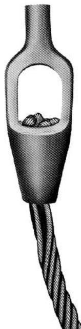
Figure 6: Insert the wire rope through the body and thread it back through the front
