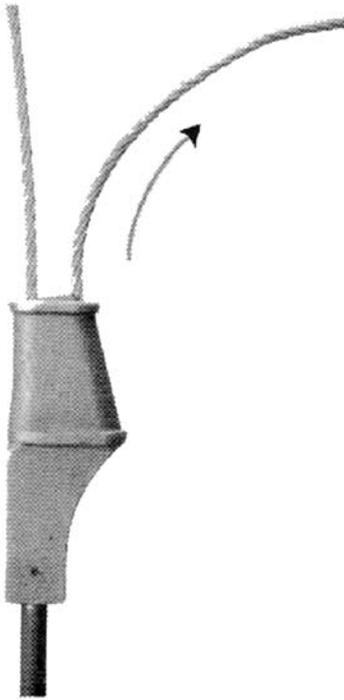
to bind the dead end to the live, or load bearing, end of the rope. Place the first clip a maximum of four times the rope's diameter above the socket, and the second clip within eight times the rope's diameter above the first clip. The purpose of the clips is to retain the wedge and prevent the rope from slipping should the load be removed for any reason.
